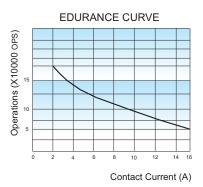
**Test conditions:**Resistive load,250VAC 85°C , 1s on 9s off
