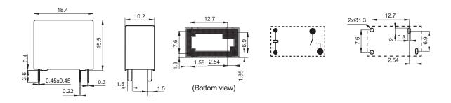
The pin dimension of the product outline drawing is the size before tinning (it will become larger after tinning), and the mounting hole size is the recommended design size of the PCB board hole. The specific PCB board hole design size can be mapped and adjusted according to the actual product.
